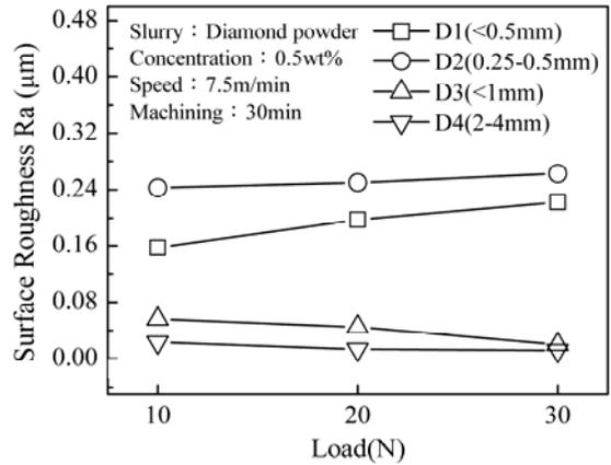
Fig. 15 Relationship between load and surface roughness
