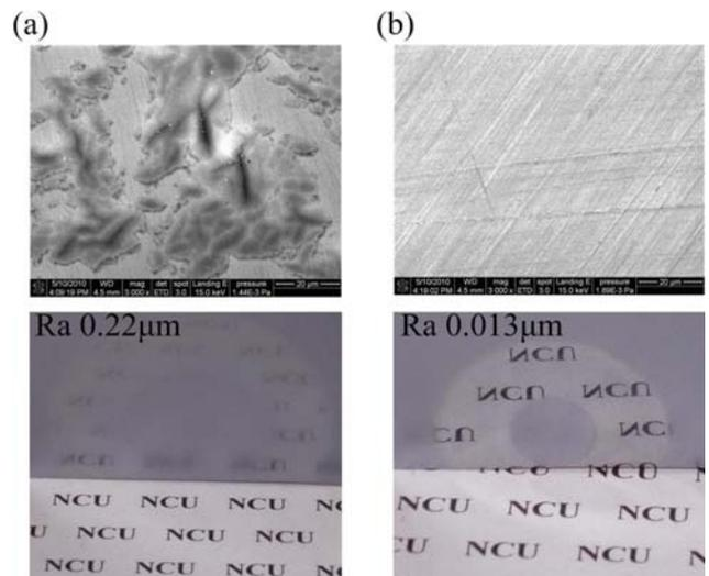
Fig. 17 Polishing by (a) D1 (b) D3 particles under conditions of machining time 30min., speed 7.5m/min. and load 30N
