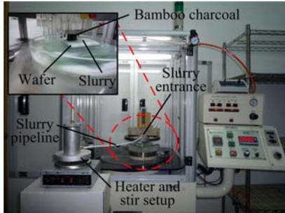
Fig. 1 Experimental equipments
