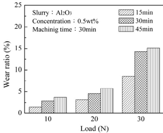
Fig. 9 Relationship between load and the wear of bamboo charcoal
