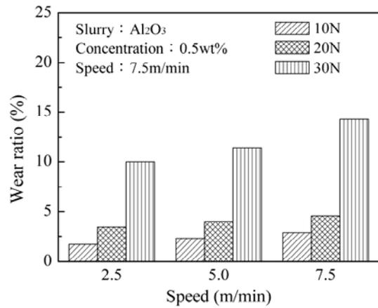
Fig. 6 Relationship between machining speed and the wear of bamboo charcoal
