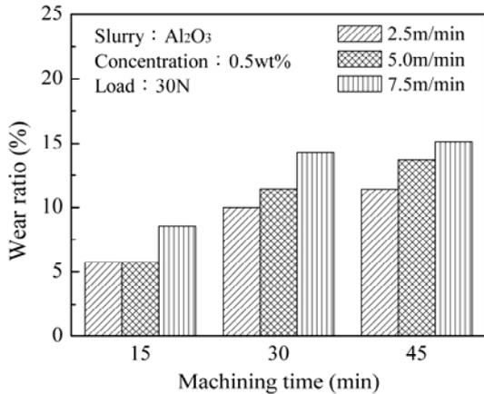
Fig. 4 Relationship between machining time and wear of bamboo charcoal
