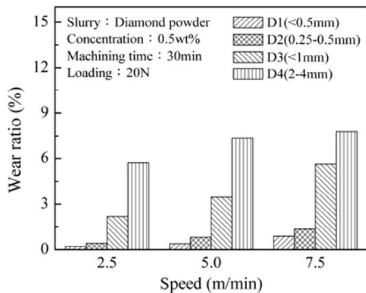
Fig. 14 Relationship between machining speed and the wear of bamboo charcoal
