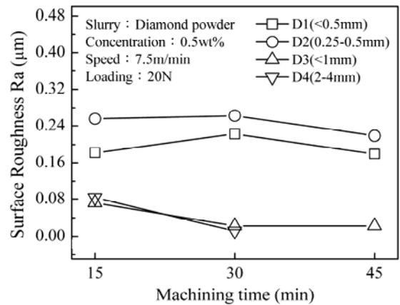
Fig. 11 Relationship between machining time and surface roughness
