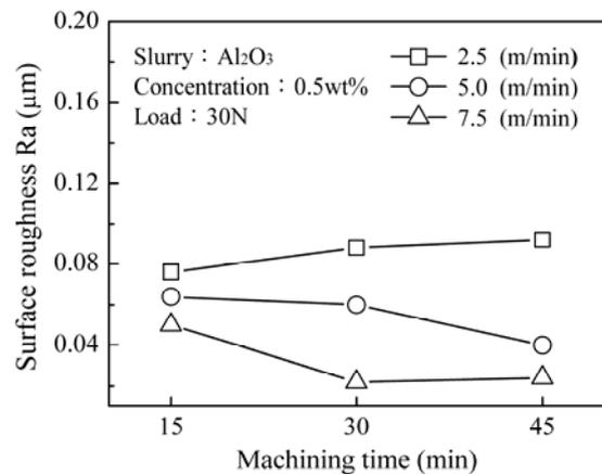
Fig. 3 Relationship between machining time and surface roughness under different speeds
