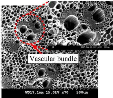
Fig. 2 Structure of bamboo charcoal
