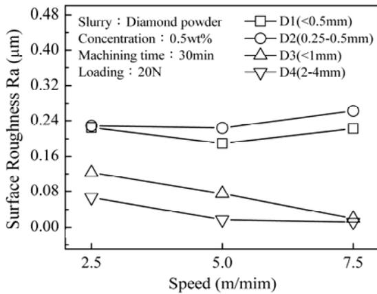
Fig. 13 Relationship between machining speed and surface roughness
