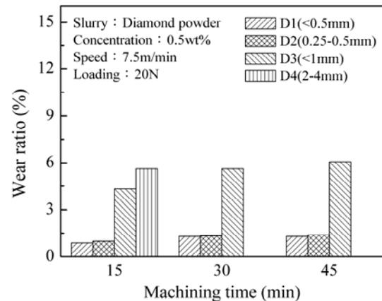
Fig. 12 Relationship between machining time and the wear of bamboo charcoal
