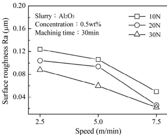
Fig. 5 Relationship between speed and surface roughness under different loads
