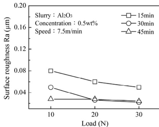
Fig. 8 Relationship between load and surface roughness under different machining time
