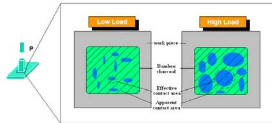
Fig. 7 Schematic diagram of applied load and actual contact area
