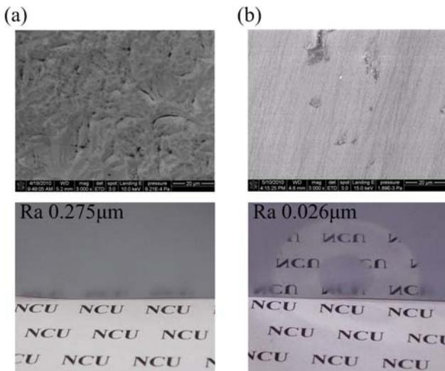
Fig. 10 Comparison of sample surfaces (a) of original sample (b) after polishing
