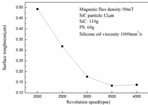
Fig. 8 Impact of Spindle Speed on Surface Roughness
