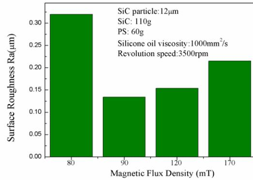
Fig. 3 Impact of Magnetic Flux Density on Surface Roughness
