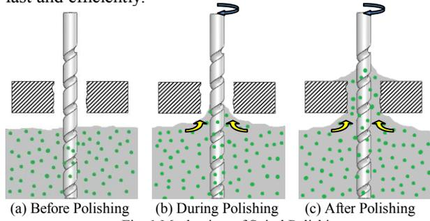
Fig. 1 Mechanism of Spiral Polishing
