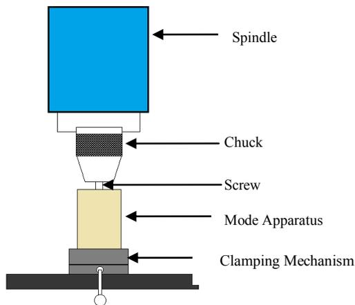
Fig. 2 Illustration of the Mold
