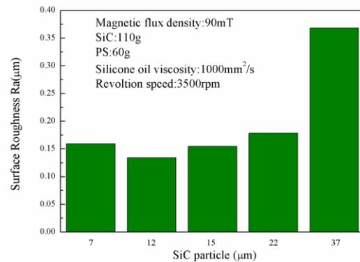
Fig. 4 Impact of SiC Grains Size on Surface Roughness
