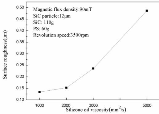
Fig. 7 Impact of Silicone Oil Viscosity on Surface Roughness
