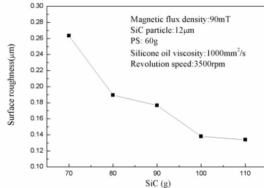
Fig. 5 Impact of SiC Grains Weight on Surface Roughness
