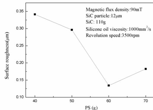
Fig. 6 Impact of PS Weight on Surface Roughness
