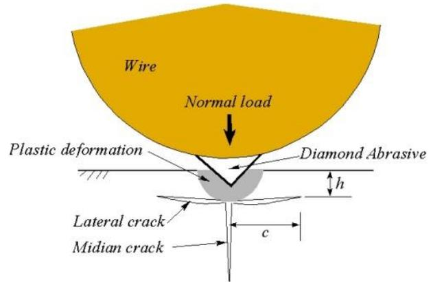
Fig. 1 Mechanism of brittle indentation fracture during fixed abrasive wire sawing.
