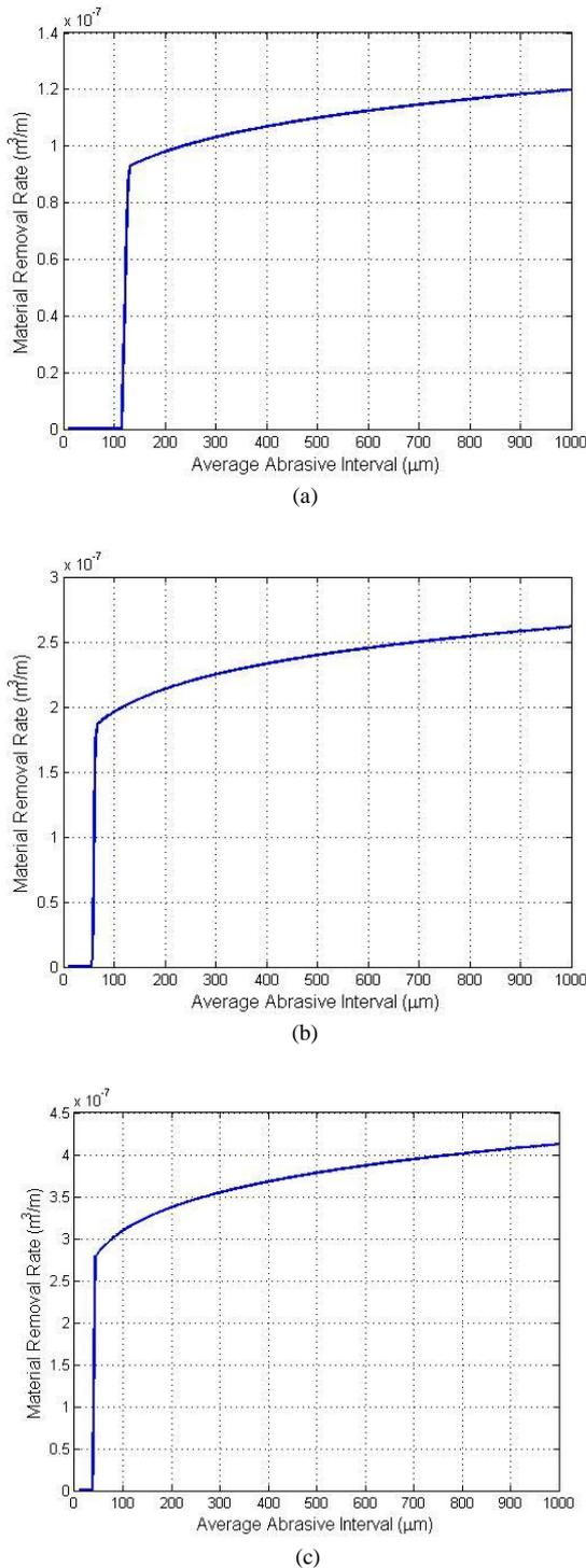
Fig. 7 Material removal rate with wire tensions (a)  $P = 10$  N, (b)  $P = 20$  N, and (c)  $P = 30$  N at the entry of slicing zone. The wire bow angle is  $b = 5^\circ$ .
