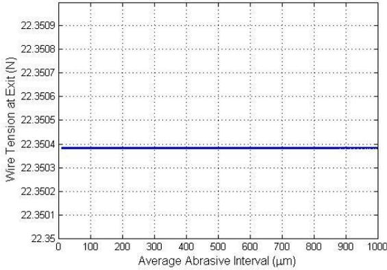
Fig. 5 Wire tension at the exit versus the variation of abrasive interval. The wire tension at the entry is 20 N, and the bow angle is  $5^\circ$ .
