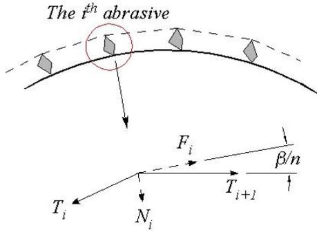
Fig. 4 Analysis of wire tension around an abrasive grit
