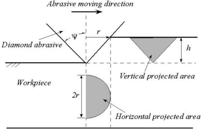
Fig. 2 Mechanism of conical abrasive wear.
