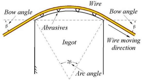
Fig. 3 Configurations of the wire and slicing groove.
