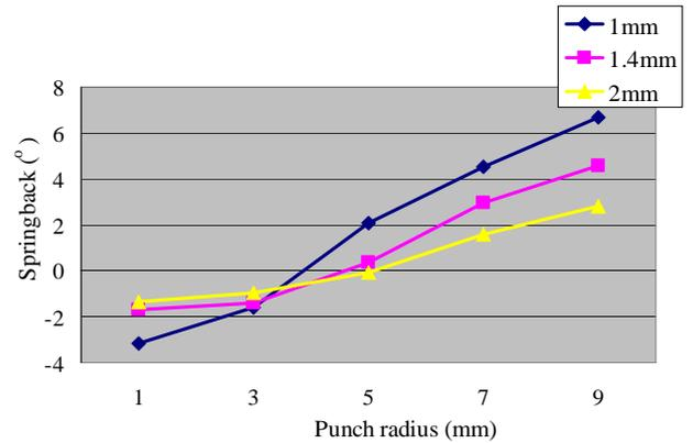
Fig. 4 Springback versus punch radius for 590Y with various thicknesses in V-bending
