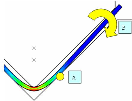
Fig. 10 Deformation of sheet metal in V-bending
