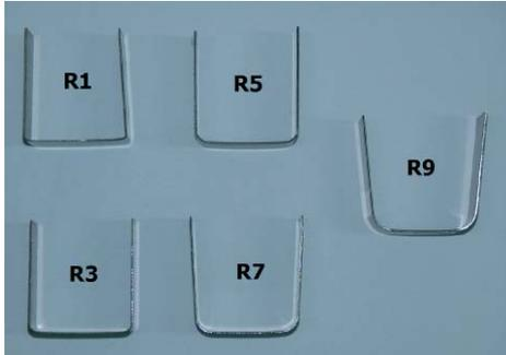
Fig. 5 Deformed shapes for 590R steel after U-bending
