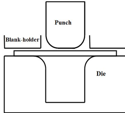
Fig. 7 Tooling used for U-hat bending
