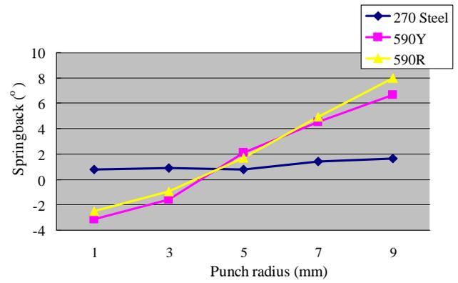
Fig. 3 Springback versus punch radius for three steels in V-bending
