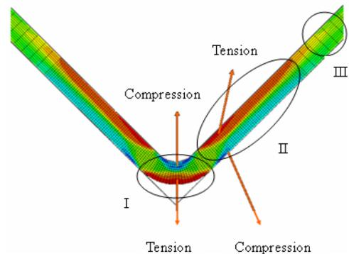
Fig. 11 Stress distribution along the sheet metal in V-bending
