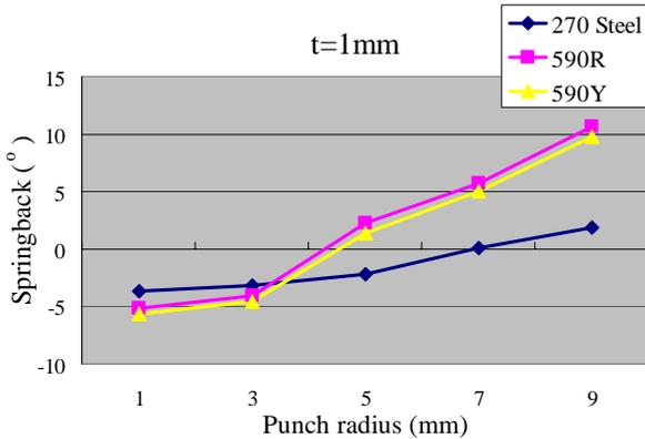
Fig. 6 Springback versus punch radius for three steels in U-bending
