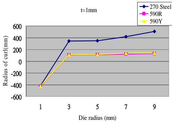
Fig. 9 Side-wall curls occurred in the U-hat bending for three steels
