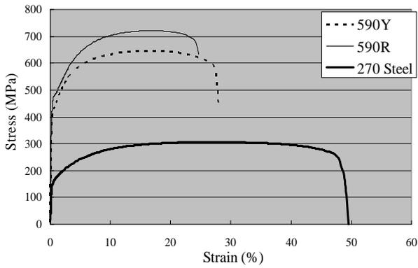
Fig. 1 Stress strain relations of three kinds of steel
