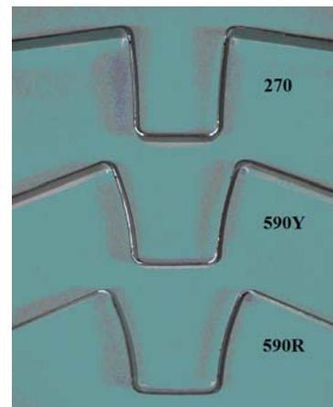
Fig. 8 Side-wall curls occurred in the U-hat bending for three steels
