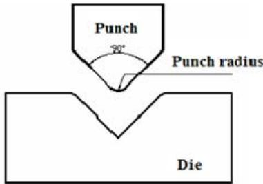
Fig. 2 Tooling used for V-bending
