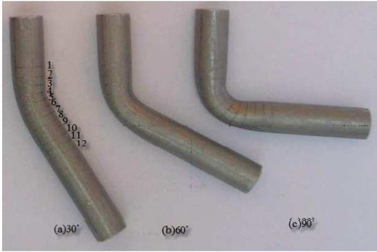
Fig. 5 Metal flow field mark and analysis (30°, 60°, 90°)
