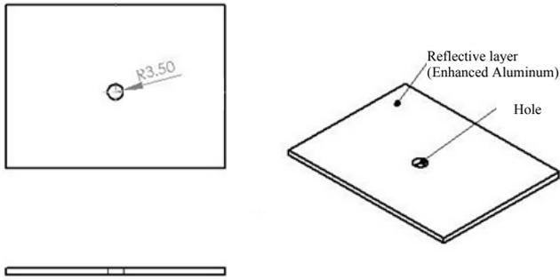
Fig. 3 Schematic diagram of the mirror with a hole
