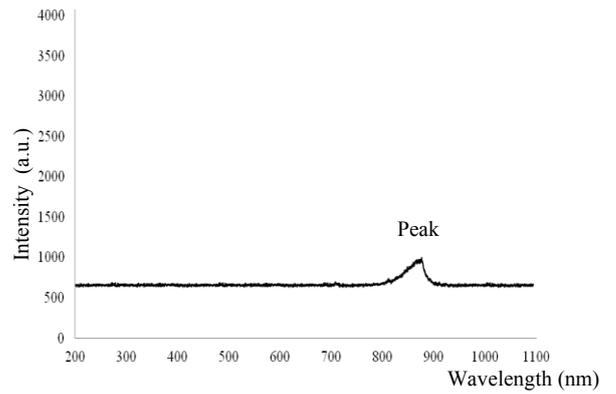
Fig. 8 The GaAs/GaAs<sub>1-x</sub>P<sub>x</sub> spectrum detected by traditional PL
