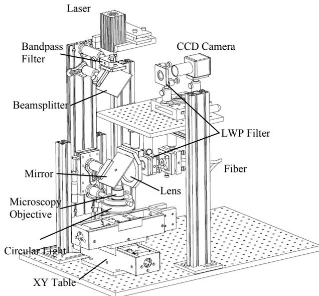
Fig. 5 Schematic diagram of the measurement system design
