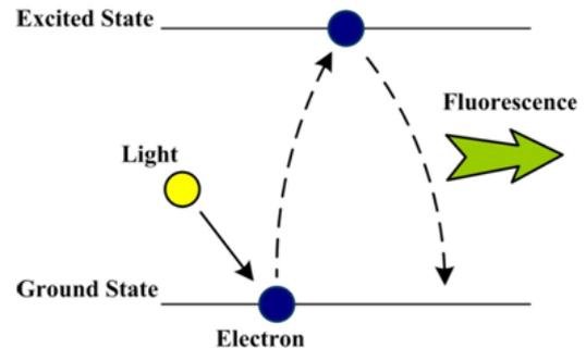
Fig. 1 Schematic diagram of PL principle
