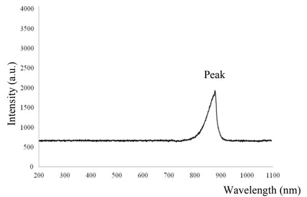
Fig. 9 The GaAs/GaAs<sub>1-x</sub>P<sub>x</sub> spectrum detected by the developed system
