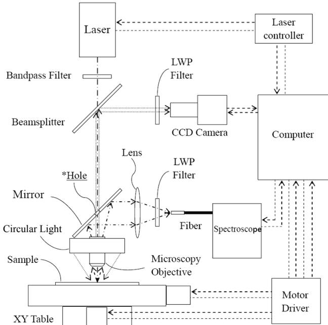
Fig. 4 Schematic diagram of the developed system
