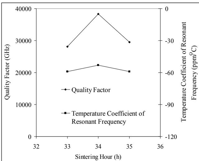
Fig. 4 Quality factor and temperature coefficient of resonant frequency of  $\text{La}_2\text{Sn}_2\text{O}_7$  ceramics sintered at  $1550\text{ }^\circ\text{C}$  for 33-35 h.
