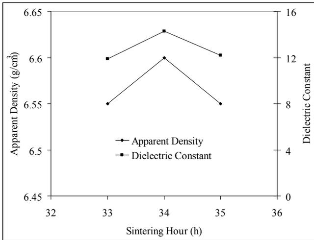
Fig. 3 Apparent densities and dielectric constant of  $\text{La}_2\text{Sn}_2\text{O}_7$  ceramics sintered at  $1550\text{ }^\circ\text{C}$  for 33-35 h.
