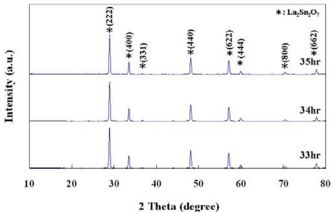
Fig. 1 X-ray diffraction patterns of  $La_2Sn_2O_7$  ceramics sintered at 1550 °C for 33-35 h.
