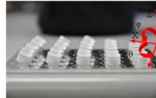
Fig 15. LED wire frame module with bent packages
