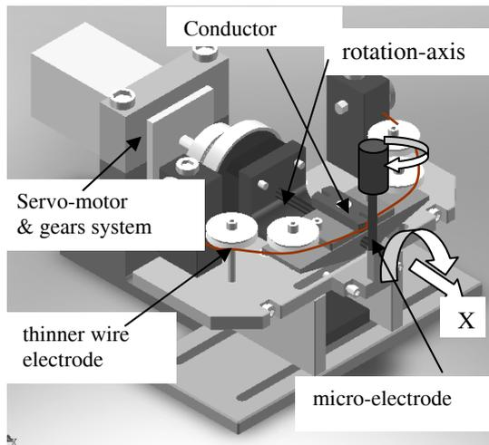
Fig. 1. Solid model of the novel design for augmented rotational axis to a general WEDG system.
