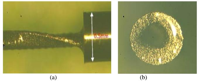
Fig. 12. Lateral view and end view for a long pitch of screw conducted by the proposed multi-axial UA-WEDG system.
