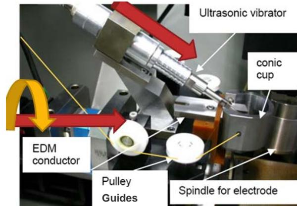
Fig. 2. Ultrasonic vibration assisted mechanism setup for the multi-axial WEDG system (UA-WEDG).
