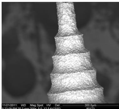
Fig. 11. SEM photo of the rod with UA-WEDG dressing into 0.1 mm diameter from 0.5 mm.
