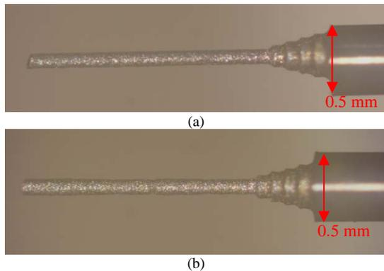
Fig. 10 Comparison of the dressing results, (a) with general standard WEDG (95 min 14 S), (b) with UA-WEDG (65 min 27 S), dressed into 100 micron dia with 1.6 mm long.
