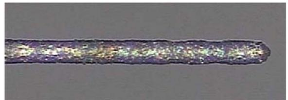
(b) Averaged diameter of 22.2 micron with on-line measurement
