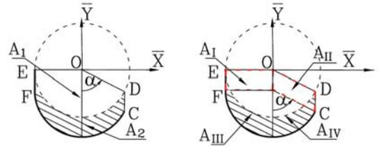
Fig. A. Computation model for sweeping area with coordinate transformation for multi-axial WEDG mechanism.
