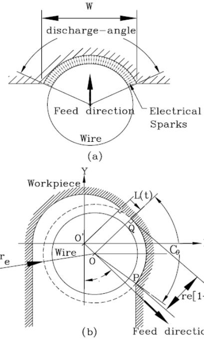
Fig. 5. (a) Definition of discharge-angle  $C_\theta$  in wire-EDM top view. (b) ideal removal model for corner cutting.
