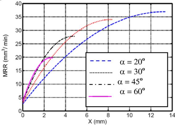
Fig. 7. Theoretical removal rates (MRR) for several inclined angles from 20° to 60°.
