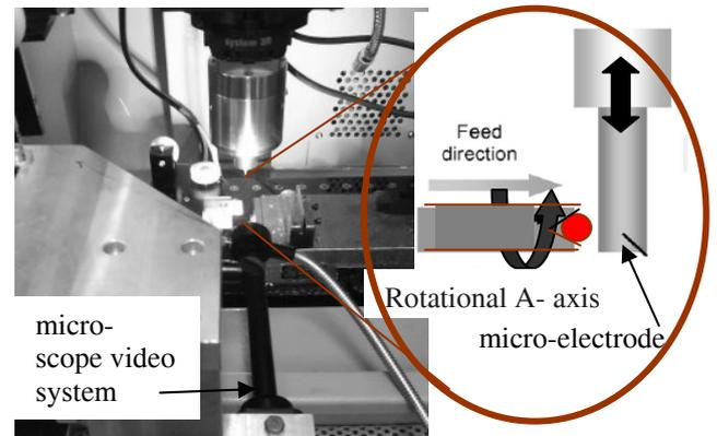
Fig. 4. Assembled multi-axial WEDG on the micro-EDM machine with microscope video system.
