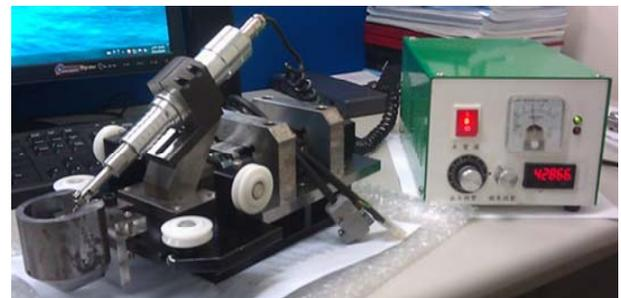
Fig. 3. Setup of the ultrasonic vibrator and its power supply.
