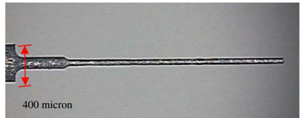
(a) Step shaft dressed by WEDG from 100 micron to 40 micron dia.
