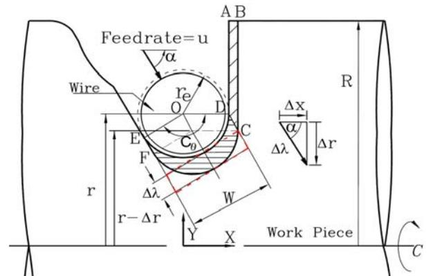
Fig. 6. General removal model for WEDG an inclined  $\alpha$  angle of wire with respect to the revolution axis.
