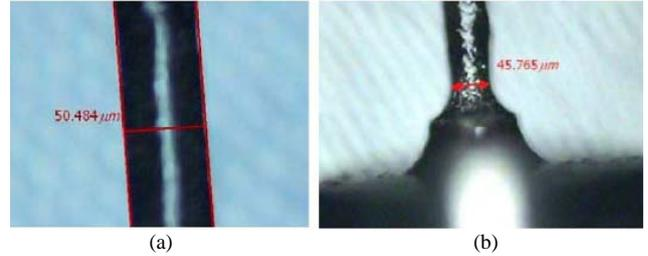
Fig 8. (a) Micro-rod of 50  $\mu\text{m}$  dia. is dressed by the proposed mechanism, and (b) its step neck near the raw material of 500  $\mu\text{m}$ .
