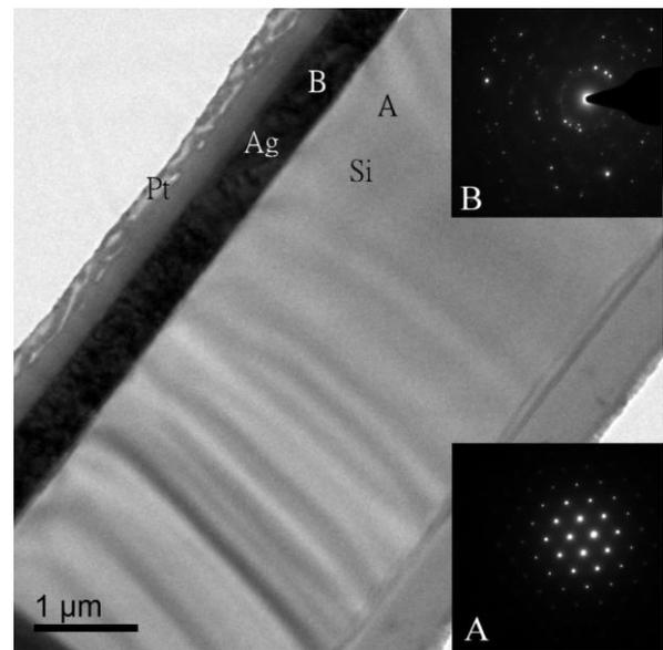
Fig. 2 Bright field TEM micrograph of as-deposited Ag/Si thin-film.
