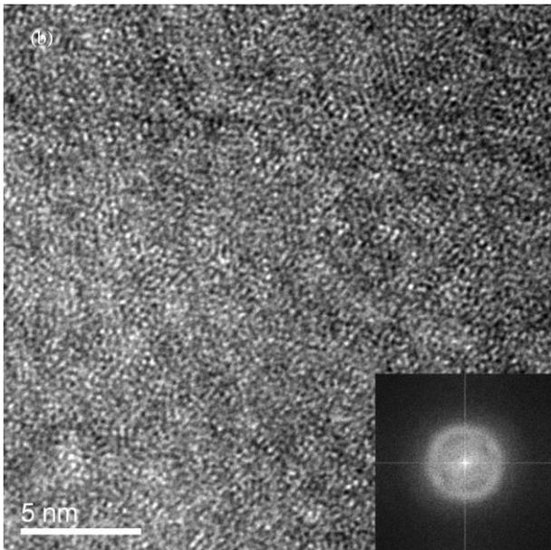
Fig. 3 (a) Bright field TEM micrograph of as-deposited indented specimen; (b) high-magnification micrograph of Si substrate; (b) high-magnification micrograph of indentation affected zone.
