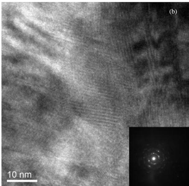
Fig. 6 (a) Bright field TEM micrograph of indented specimen annealed at 800°C for 2 min; (b) high-magnification micrograph of region B in Fig. 6(a).
