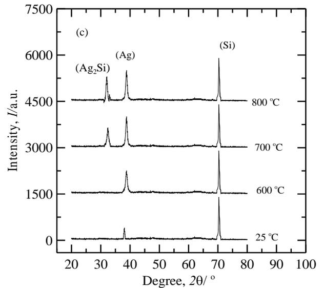
Fig. 5 (a) Bright field TEM micrograph of indented specimen annealed at 700 °C for 2 min; (b) high-magnification micrograph of indentation affected zone; (c) X-ray diffraction spectra of Ag/Si thin film at 25°C and various annealing temperatures ranging from 600°C~800°C.
