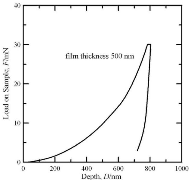
Fig. 1 Loading-unloading curve obtained during nanoindentation of as-deposited Ag/Si thin film.
