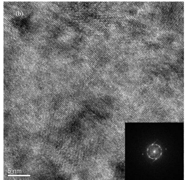
Fig. 4 (a) Bright field TEM micrograph of indented specimen annealed at 600°C for 2 min; (b) high-magnification micrograph of indentation affected zone.
