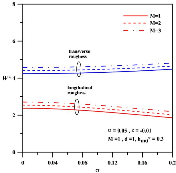
Fig. 5 Relation between  $W^*$  and  $\sigma$  with different  $M$
