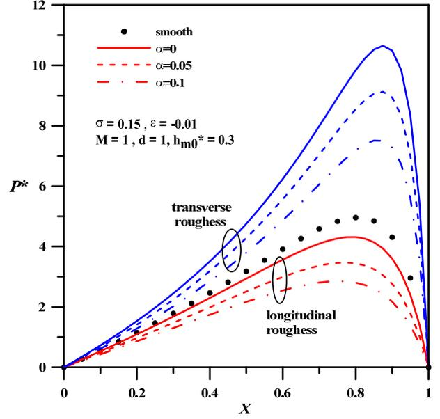
Fig. 2 Film pressure  $P^*$  as function of  $X$  for varied  $\alpha$
