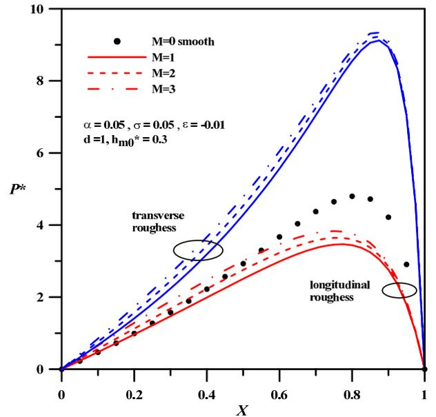
Fig. 3 Effects of magnetism  $M$  to film pressure  $P^*$
