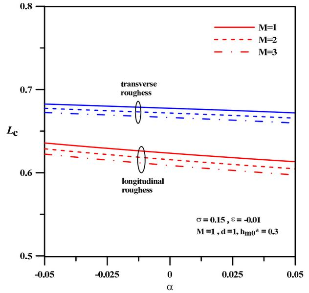
Fig. 6 Relation between  $L_c$ , and  $\alpha$  with different  $M$
