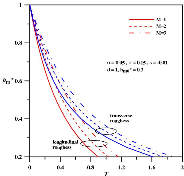
Fig. 8 Film thickness  $h_m^*$  as function of  $T$  with different  $M$
