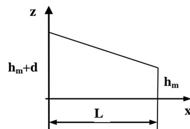
Fig. 1 Physical configuration of squeeze tilted bearing
