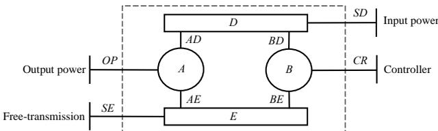
Fig. 2 Structure of series-type ICT.
