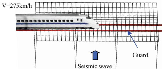
Fig. 12 A Shinkansen car on the ladder track with guard
