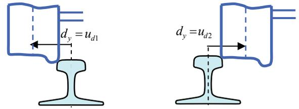
(a) Field-side derailment (b) Gauge-side derailment
