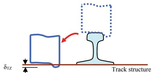
Fig. 4 Vertical relative displacement between wheel and track structure  $\delta_{TZ}$
