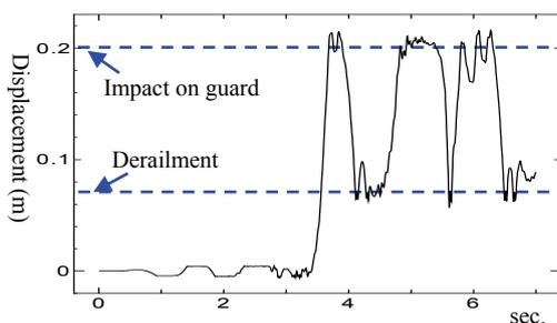
Fig. 15 Relative displacement between the right wheel and rail in the transverse direction
