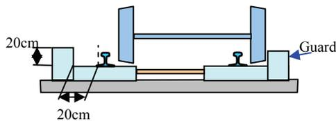
Fig. 13 Cross section of the ladder track with guard attached
