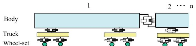
Fig. 1 Mechanical model of a Shinkansen train
