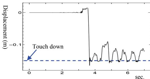
Fig. 14 Vertical displacement of the right wheel of the 1st wheel-set
