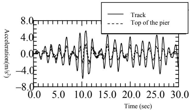
Fig. 10 Transverse acceleration response of pier P3
