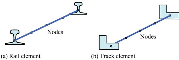
Fig. 6 Rail and track elements "
