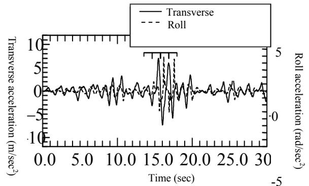
Fig. 11 Transverse and roll accelerations of the car body at the 1st car
