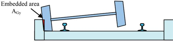
Fig. 5 Contact-impact between wheel and guard on the track structure in the transverse direction
