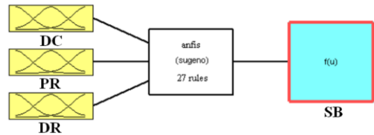
System ANAFIS: 3 input, 1 output, 27 rules Fig. 6. Fuzzy rule architecture of ANFIS model.
