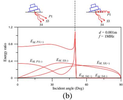
Fig. 4 Wave characteristics of incident  $P$ -wave with  $d=0.001\text{m}$  and  $1\text{MHz}$ : (a) media 1 and 3; (b) intermediate microporous plate.
