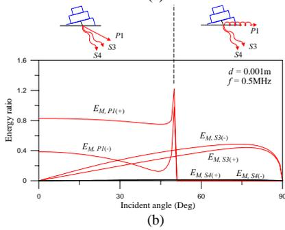
Fig. 3 Wave characteristics of incident  $P$ -wave with  $d=0.001\text{m}$  and  $0.5\text{MHz}$ : (a) media 1 and 3; (b) intermediate microporous plate.
