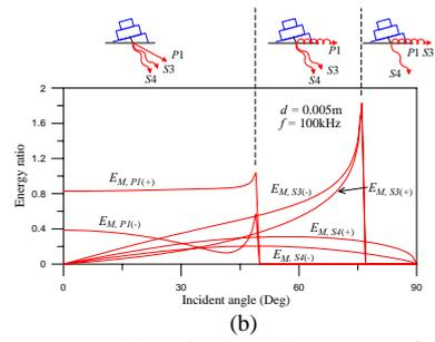
Fig. 5 Wave characteristics of incident  $P$ -wave with  $d=0.005\text{m}$  and  $100\text{kHz}$ : (a) media 1 and 3; (b) intermediate microporous plate.
