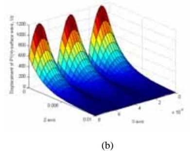
Fig. 7 Displacement of  $P1(+)$ -surface wave as function of  $x$ -axis and  $z$ -axis at  $\theta_i = 60^\circ$  and  $0.5\text{MHz}$ : (a)  $U_x$ ; (b)  $U_z$ .
