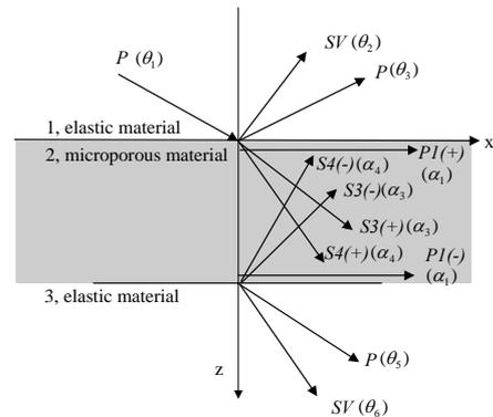
Fig. 1 Wave fields of the microporous plate placed between two elastic semi-infinite media 1 and 3.
