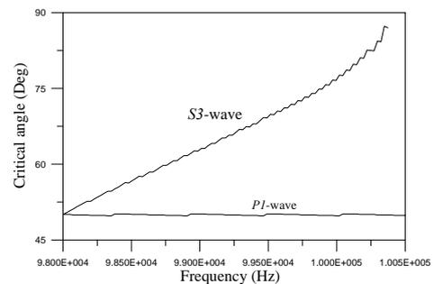
Fig. 2 Critical angles of grazing  $P1$  and  $S3$ -surface waves as the function of frequency.
