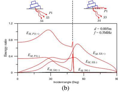
Fig. 6 Wave characteristics of incident  $P$ -wave with  $d=0.005\text{m}$  and  $0.5\text{MHz}$ : (a) media 1 and 3; (b) intermediate microporous plate.
