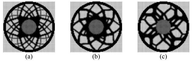
Figure 6 The topology layout of the flywheel rotor with an objective of maximizing the rotor stiffness and kinetic energy; (a) 0 RPM; (b) 1000 RPM; (c) 5000 RPM
