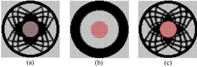
Fig. 2 Comparison of topology layouts: topology layout of maximizing (a) the fundamental torsional frequency; (b) the moment of inertia and (c) the fundamental torsional frequency and the moment of inertia
