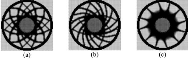
Figure 4 The topology layout of the flywheel rotor with an objective of maximizing the rotor stiffness; (a) 0 RPM; (b) 1000 RPM; (c) 5000 RPM
