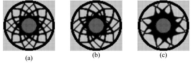
Figure 5 The topology layout of the flywheel rotor with an objective of maximizing the rotor stiffness; (a) 0 RPM; (b) 1000 RPM; (c) 5000 RPM
