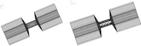
Fig. 3 CFD modelling diagram of the abrasive medium without/with a helical passageway.
