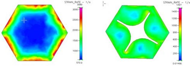
(a) Hexagon hole without mold core (b) Hexagon hole with a helical core
