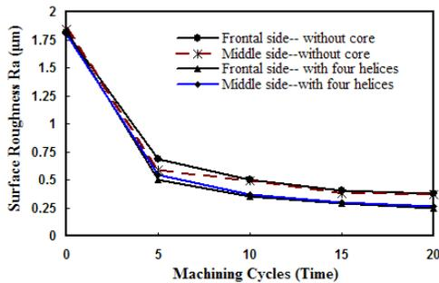
Fig. 14 The distribution diagram of surface roughness in octagon without/with four helices core.
