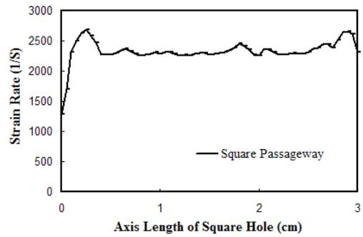
Fig. 6 The curve diagram of axial strain-rate in a square passageway.
