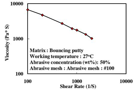
Fig. 1 Shear rates Effects on viscosities.
