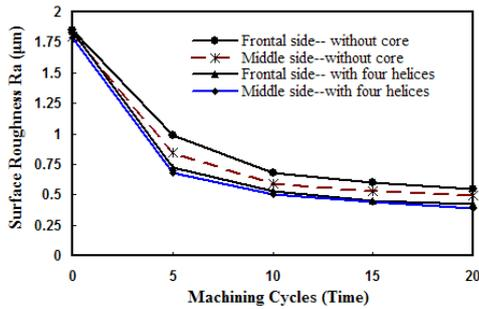
Fig. 13 The distribution diagram of surface roughness in square without/with four helices core.
