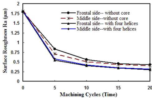
Fig. 14 The distribution diagram of surface roughness in hexagon without/with four helices core.
