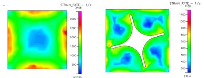
(a) Square hole without mold core (b) Square hole with four helices core
