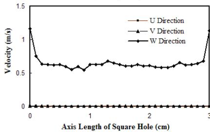
Fig. 4 The curve diagram of axial velocity in a square passageway.
