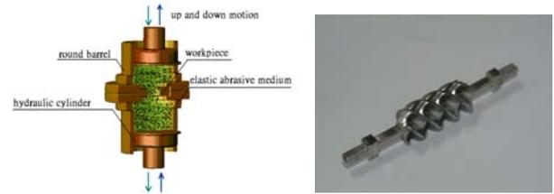
(a) Machining process of AFM
