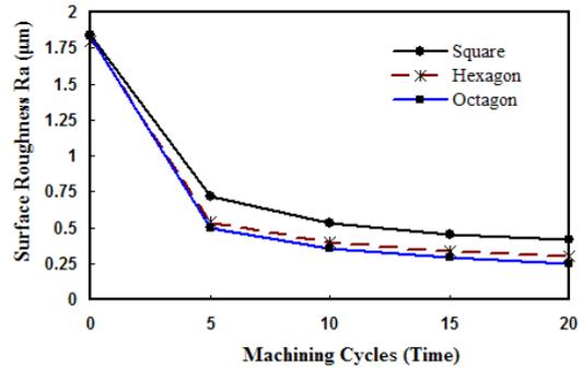
Fig. 12 The distribution diagram of surface roughness in different polygon passageway with a four helices core.
