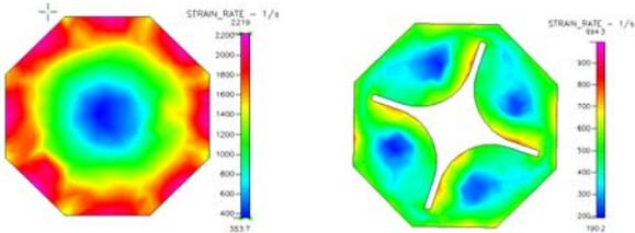
(a) Octagon hole without a mold core (b) Octagon hole with a helical core
