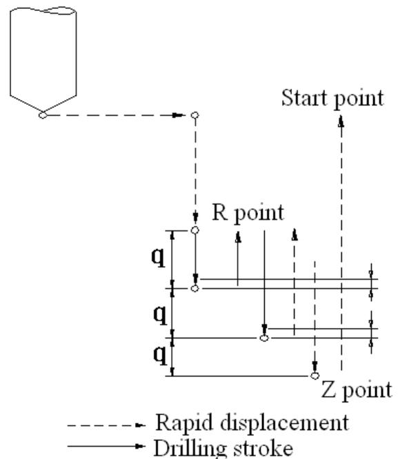
Fig. 2 Illustration of G83 (peck drilling cycle)
