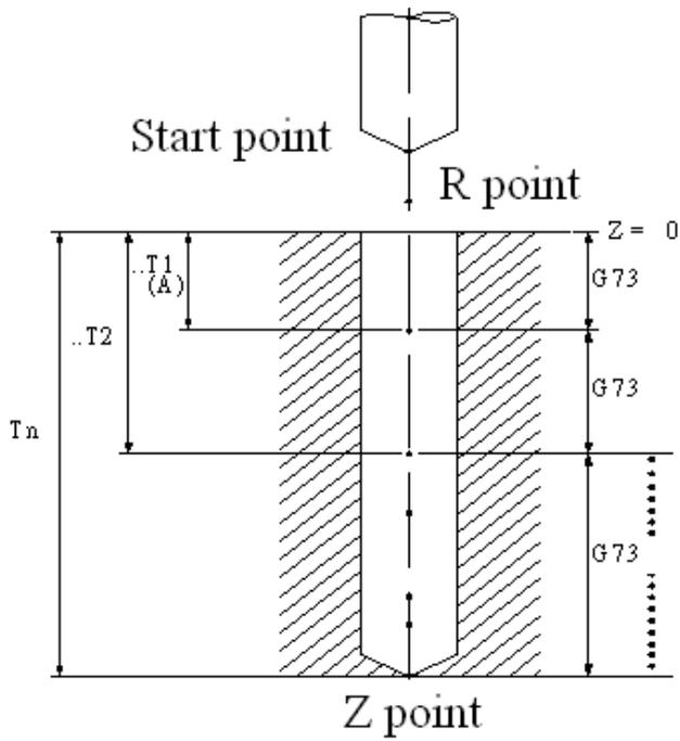
Fig. 3 Illustration of the hybrid command of deep hole drilling G251
