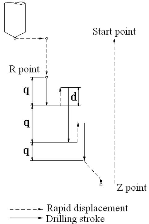
Fig. 1 Illustration of G73 (high-speed peck drilling cycle)
