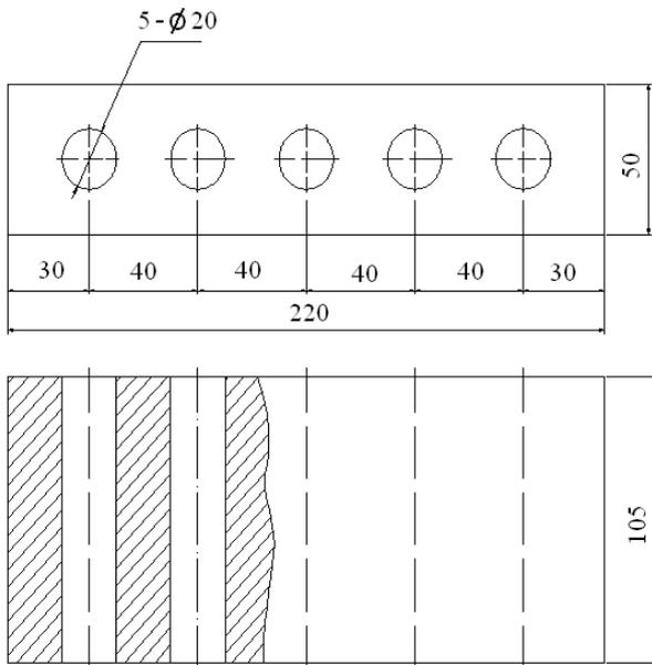
Fig. 4 The drawing of workpiece
