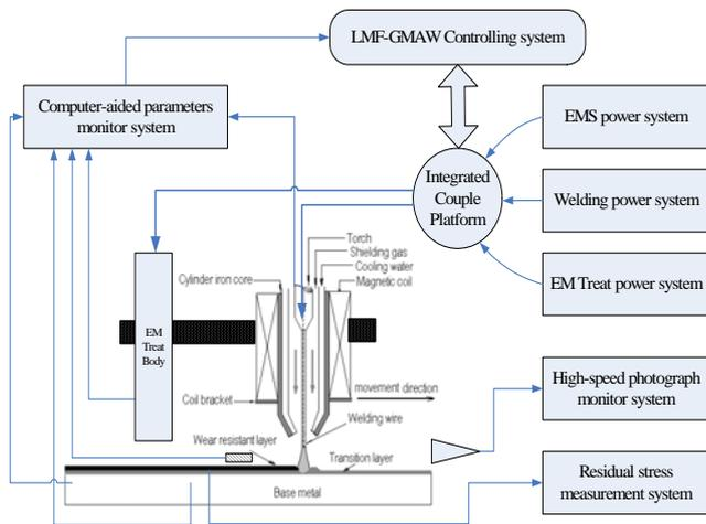
Fig. 1 Principle of LMF-GMAW welding system.
