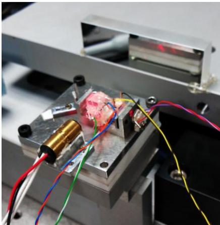
Fig. 6 The photo of the miniature interferometer
