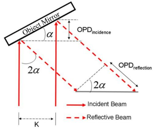
Fig. 3 Optical path difference caused by angle displacement
