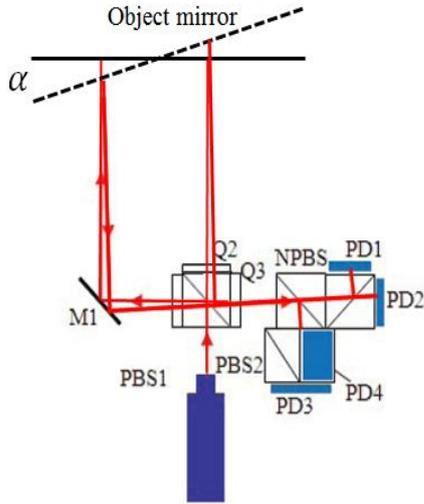
Fig. 2 The movement of reflected beam
