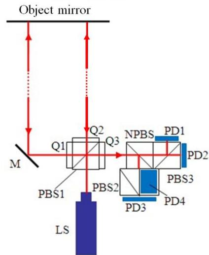
Fig. 1 Structure of Michelson angle interferometer (LS: laser diode, PBSi: ith polarizing beam splitter, M: mirror, NPBS: non-polarizing beam splitter, Qi: ith quarter waveplate, PDi: ith photodetector.)
