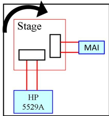
Fig. 7 Calibration system
