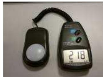
Fig. 4-4 The illumination measured without diffractive optical element
