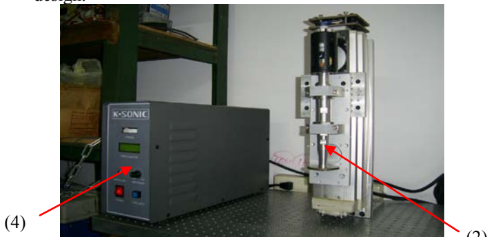
Figure 6 Vertical installation of the vibration equipment group
