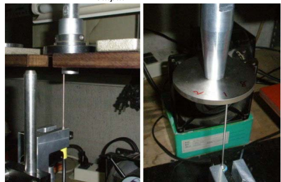
Figure 8 Measurement of displacements at input/output ends of the horn
