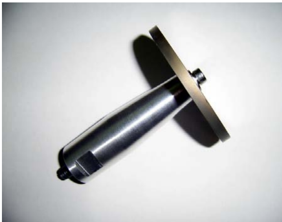
Figure 4 Finished product by optimal design of disc-coupled uniform section cone-shaped horn
