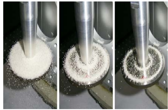
Figure 7 Pitch circles of vibration disc
