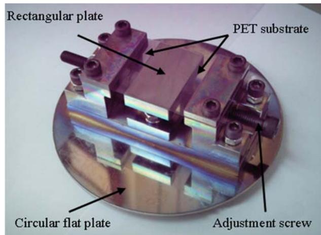
Fig. 1 Photograph of mold used to produce strain on PET substrate fixed on the rectangular area.
