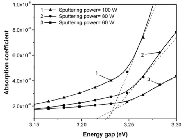
Fig. 5 Energy gaps of AZO films on a pre-strained substrate with various sputtering powers.
