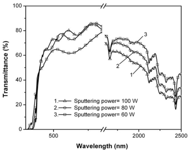
Fig. 4 Transmittance of AZO films on a pre-strained substrate with various sputtering powers.
