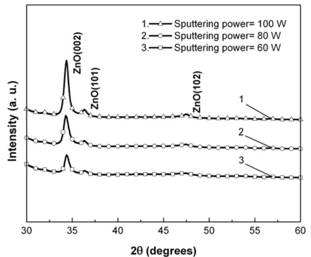
Fig. 2 XRD patterns of AZO thin film for various sputtering powers.
