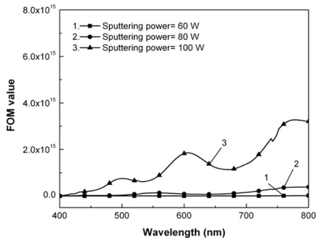
Fig. 7 FOM values of AZO films on a pre-strained substrate with various sputtering powers.
