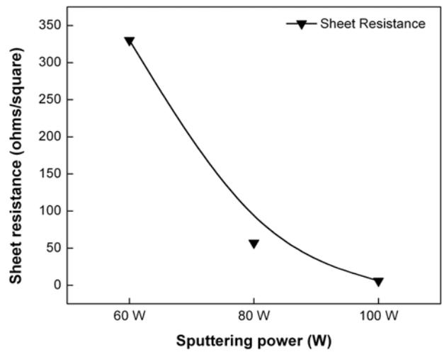
Fig. 6 Sheet resistances of AZO films on a pre-strained substrate with various sputtering powers.
