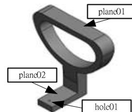
Fig. 1 Features of Arm Rest Component
