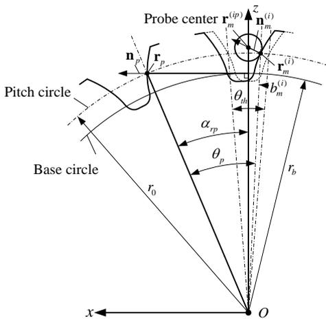
Fig. 7 Pitch deviation measurement.
