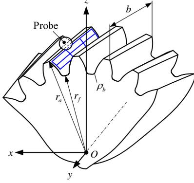
Fig. 8 The flank topographic measurement.
