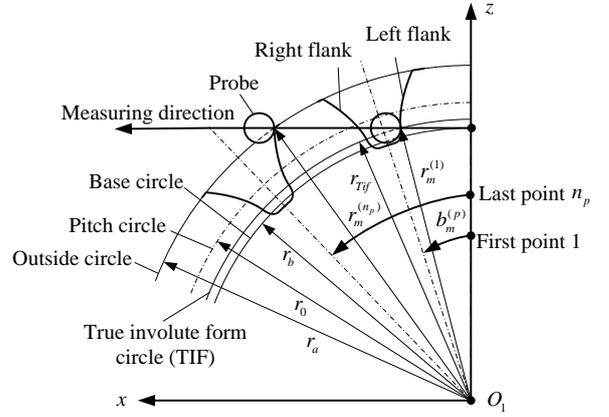
Fig. 3 Profile deviation measurement.
