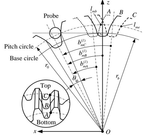
Fig. 6 Lead deviation measurement.
