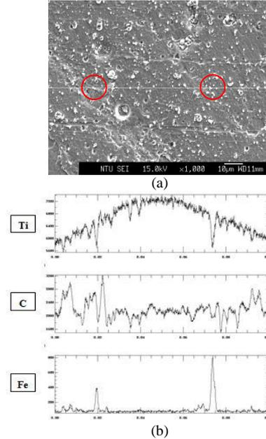
Fig. 3 FC25/TiC specimen (a)Top-view. (b) Line-scan result.
