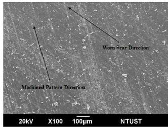
Fig. 9 Worn surface of FC25/N.
