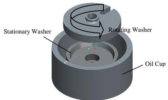
Fig. 1 Schematic diagram of a thrust washers sliding contact.
