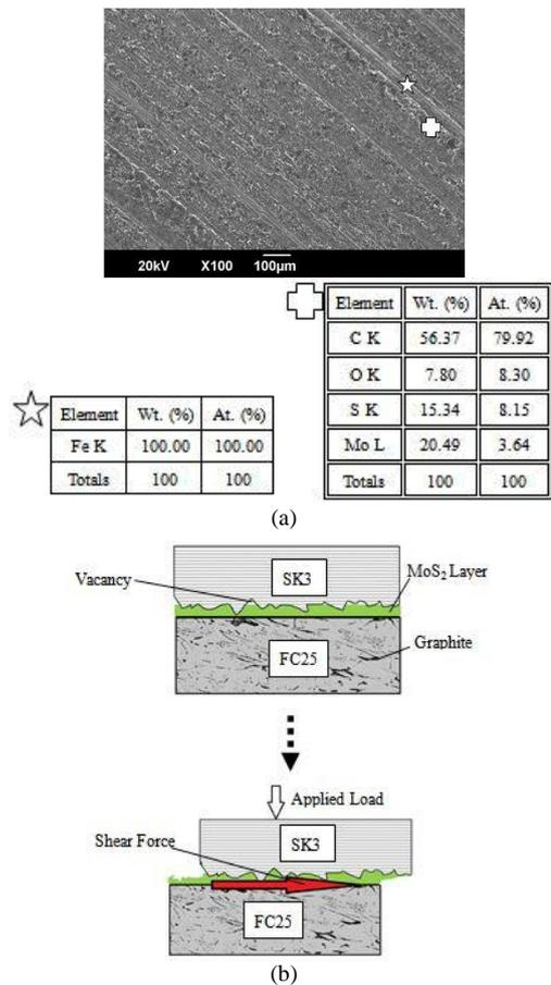
Fig. 10 FC25/MoS<sub>2</sub> wear specimen (a) Worn surface and EDS result. (b) Schematic diagram of MoS<sub>2</sub> layer deformation process during wear test.
