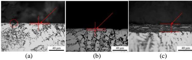
Fig. 2 Cross-section of (a) FC25/TiC. (b) FC25/N. (c) FC25/MoS<sub>2</sub> specimen.
