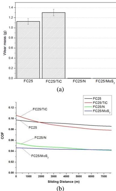
Fig. 6 Various specimens (a) Wear loss. (b) Friction coefficient.
