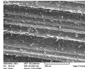
Fig. 7 Worn surface of FC25 specimen.
