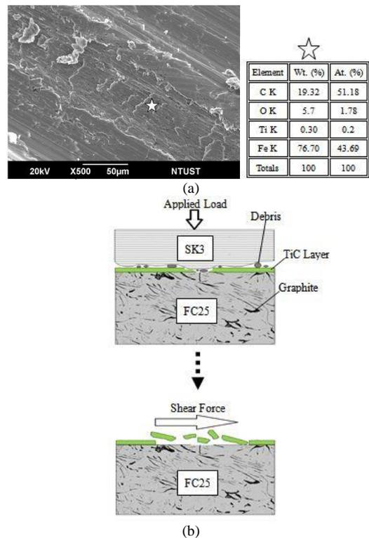
Fig. 8 FC25/TiC wear specimen (a) Worn surface and EDS result. (b) TiC film peeling-off schematic diagram.
