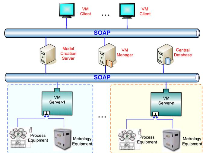
Fig. 1 An equipment monitoring system with AVM capabilities [5].
