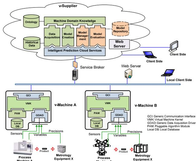
Fig. 2 Architecture of the proposed cloud computing-based intelligent equipment monitoring system.
