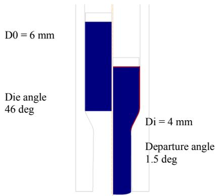
Fig. 8 Forward extrusion simulation setup
