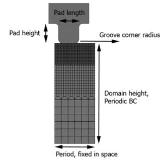
Fig. 1 Mesoscale simulation setup
