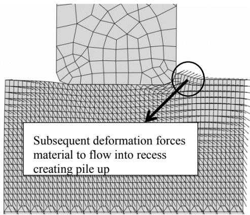
Fig. 4 Material flow in mesoscale simulation
