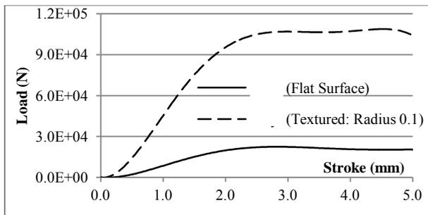
Fig. 9 Process load from extrusion simulations
