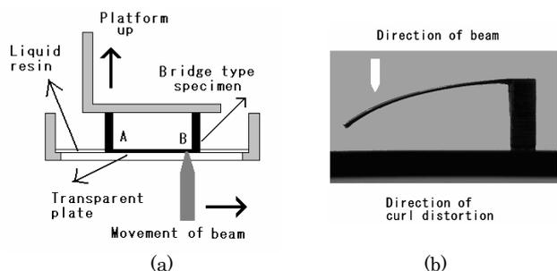
Fig. 5 Machine E-DARTS as COLAMM system. Cantilever specimen (b) is set upside down after cutting a corner A or B of bridge type specimen (a).
