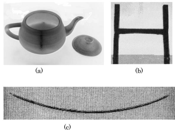
Fig. 1 3-dimensional models (a), (b) produced by SL process and a single strand (c) created by exposure of ray.
