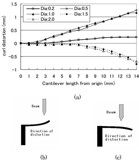
Fig. 4 Distribution of curl distortion of cantilever specimen in experiments. Direction is shown in a case (b) where diameters are 0.5 and 1.0mm, and (c) where diameters are 1.5 and 2.0mm.
