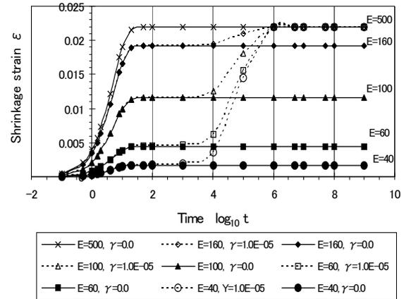
Fig. 3 Shrinkage strain  $\epsilon$  - time  $t$  curves depending on exposure energy  $E$  [ $\text{mJ}/\text{cm}^2$ ]. Number of second is 3600s for an hour,  $8.64 \times 10^4$ s for a day,  $6.05 \times 10^5$ s for a week,  $2.59 \times 10^6$ s for a month,  $3.15 \times 10^7$ s for a year, and  $3.15 \times 10^8$  s for 10 years.
