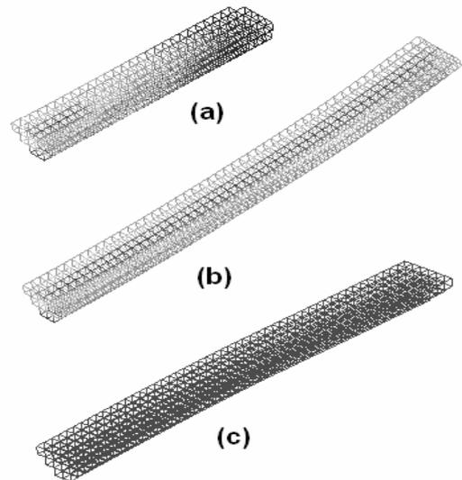
Fig. 9 Deformation and formation of cured resin produced by irradiation of u. v. ray.
