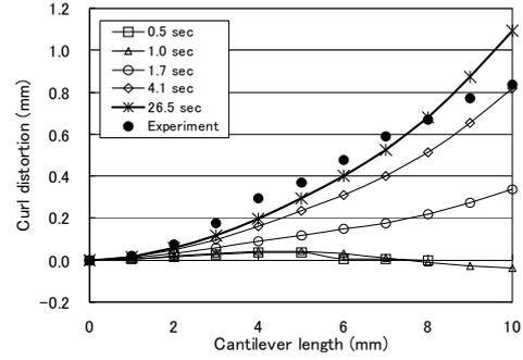
Fig. 8 Numerical result of curl distortion compared with experimental data when  $\gamma=0.0$  sec<sup>-1</sup>
