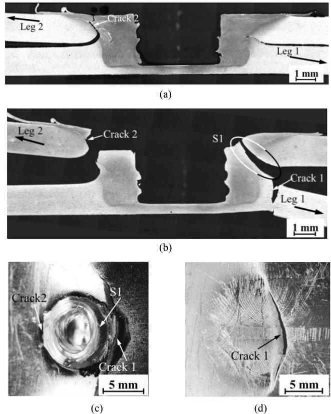
Fig. 6(a) A micrograph of the symmetry cross section of a partially failed swept spot friction weld at the fatigue life of  $2 \times 10^3$  cycles, (b) A micrograph of the symmetry cross section of a failed swept spot friction weld at the fatigue life of  $4.5 \times 10^3$  cycles, (c) a top view of a swept spot friction weld on the lower sheet of a failed specimen, (d) a back view of a swept spot friction weld on the lower sheet of a failed specimen.
