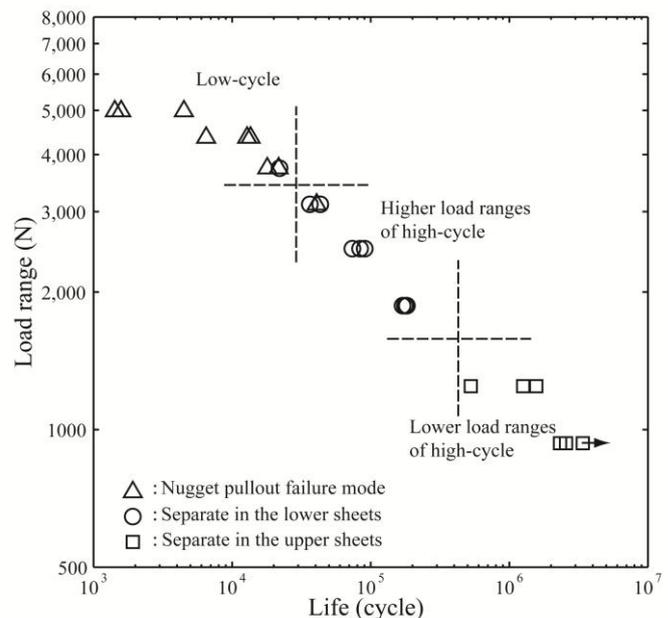
Fig. 3 Experimental results of swept spot friction welds in lap shear specimens under cyclic loading conditions.
