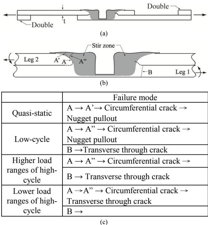
Fig. 4 (a) A schematic plot of the symmetry cross section of a lap-shear specimen made by the concave tool with the sheet thickness  $t$  under an applied force (shown as bold arrows), (b) a schematic plot of the cross section near the swept spot friction weld, (c) the failure modes of swept spot friction welds under different loading conditions.
