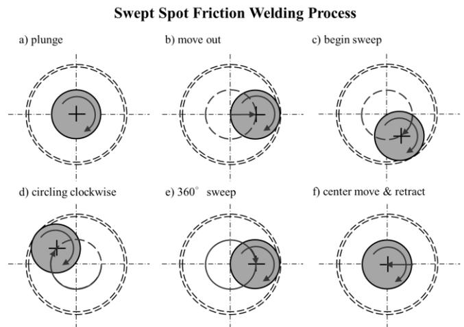
Fig. 1 A schematic of the circular tool path.
