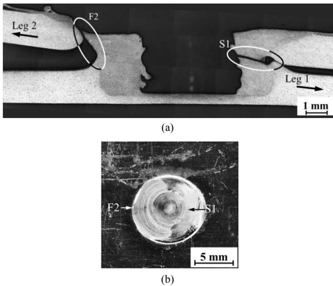
Fig. 5(a) A micrograph of the cross section of a failed swept spot friction weld under quasi-static loading conditions, (b) a top view of a swept spot friction weld on the lower sheet of a failed specimen.
