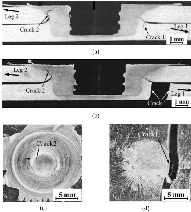
Fig. 7(a) A micrograph of the symmetry cross section of a partially failed swept spot friction weld at the fatigue life of  $6 \times 10^4$  cycles, (b) A micrograph of the symmetry cross section of a failed swept spot friction weld at the fatigue life of  $9 \times 10^4$  cycles, (c) a top view of a swept spot friction weld on the upper sheet of a failed specimen, (d) a back view of a swept spot friction weld on a failed specimen.
