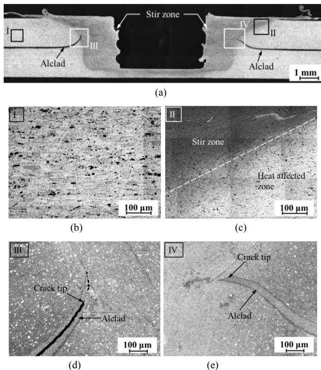
Fig. 2(a) An optical micrograph of the cross section along the symmetry plane of a swept spot friction weld, (b) a close-up optical micrograph of region I, (c) a close-up optical micrograph of region II, (d) a close-up scanning electron micrograph of region III, (e) a close-up scanning electron micrograph of region IV.
