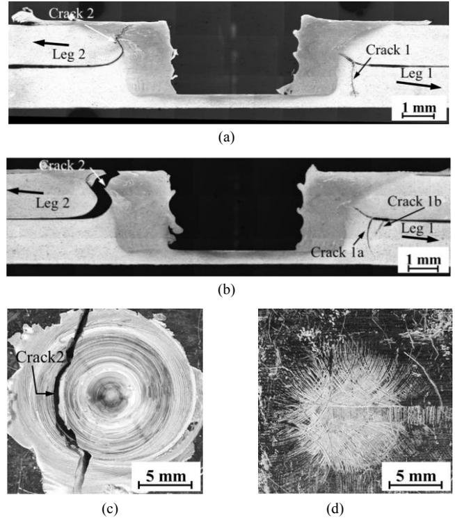
Fig. 8(a) A micrograph of the symmetry cross section of a partially failed swept spot friction weld at the fatigue life of  $10^6$  cycles, (b) A micrograph of the symmetry cross section of a failed swept spot friction weld at the fatigue life of  $1.6 \times 10^6$  cycles, (c) a top view of a swept spot friction weld on a failed specimen, (d) a back view of a swept spot friction weld on a failed specimen.
