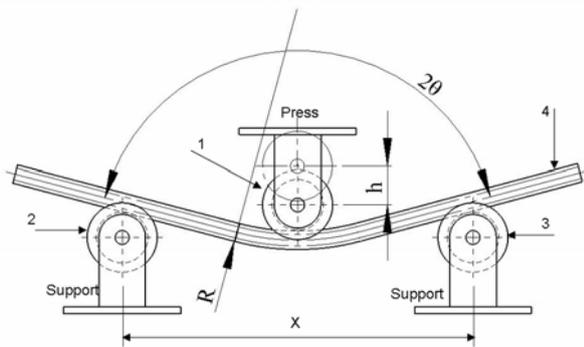
Fig. 1 Illustration of the microtube press bending principle.
