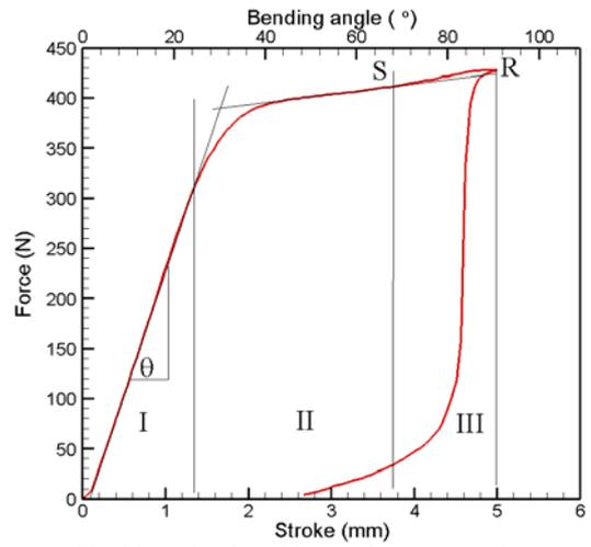
Fig. 7 Reaction force history of press vs. stroke.
