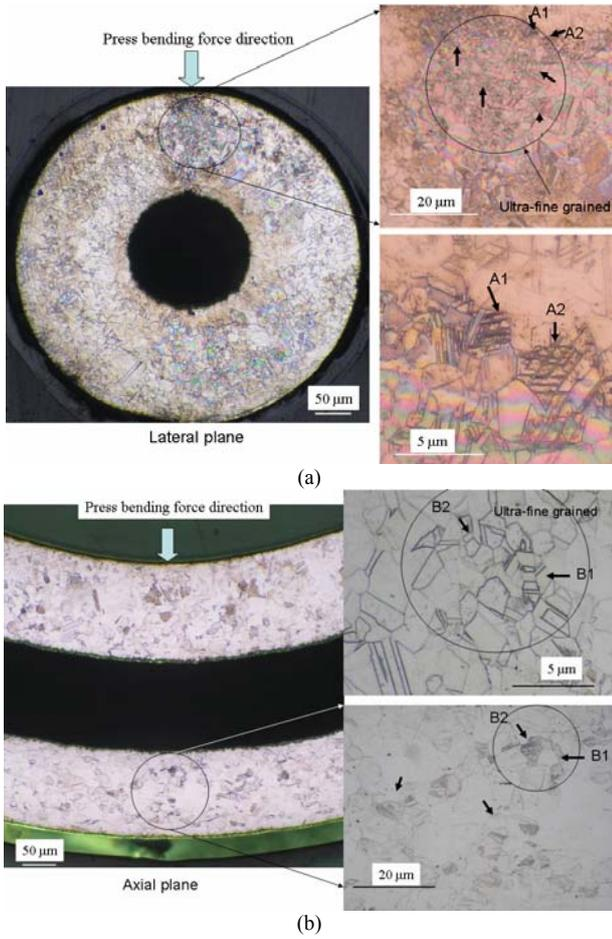
Fig. 6 Microstructure of batch AT4. (a) Microstructure of lateral plane and (b) Microstructure of axial plane.
