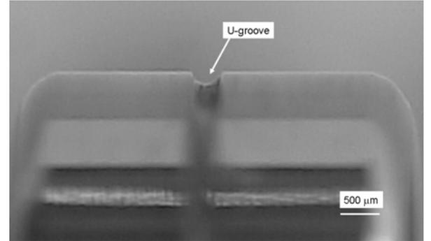
Fig.3 Bearing with U-groove (radius: 300  $\mu\text{m}$ ).
