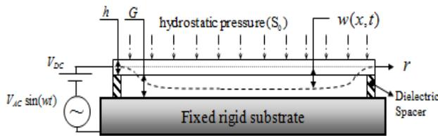
Fig. 1. Schematic illustration showing electrostatic actuation of micro circular plate.
