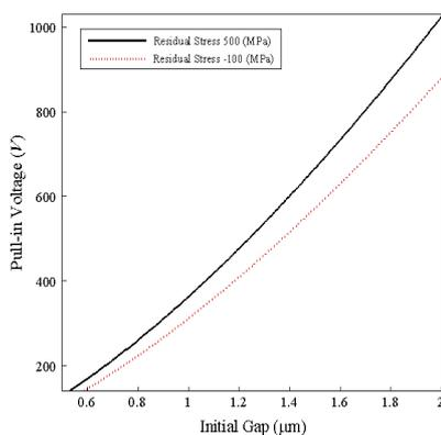
Fig. 2. Variation of pull-in voltage with initial gap height as function of residual stress
