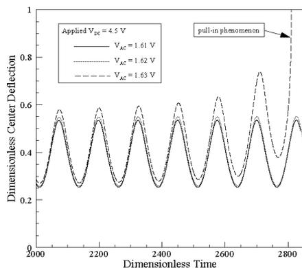
Fig. 4. Variation of dimensionless center-point displacement over time for AC voltages of 1.61 V, 1.62 V and 1.63 V, respectively. (Note that DC voltage = 4.5 V and  $\bar{\omega} = 1$ .)
