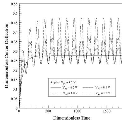
Fig. 3. Variation of dimensionless center-point displacement over time as function of AC voltage. (Note that DC voltage = 4.5 V and  $\bar{\omega} = 1$ .)
