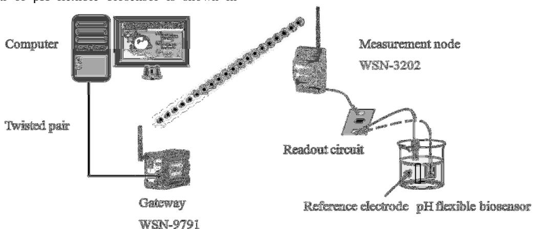
Figure 3: Schematic diagram of wireless sensing system.
