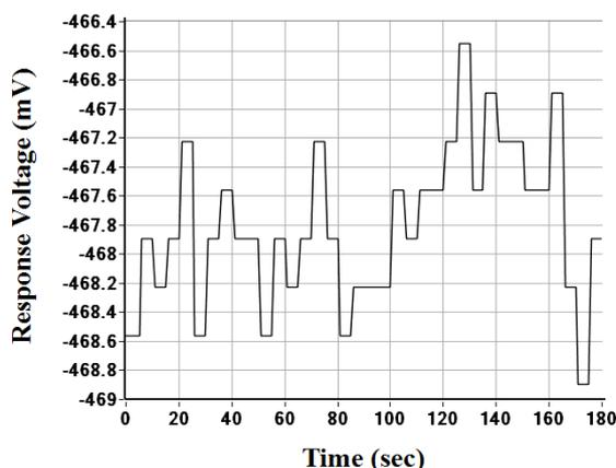
Figure 8: Measurement curve of the pH detection system with pH 3 buffer solution.
