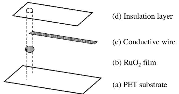
Figure 2: pH flexible biosensor cross-sectional view [13].
