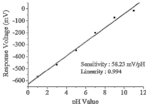
Figure 9: Diagram of measurement results of the pH flexible biosensor.
