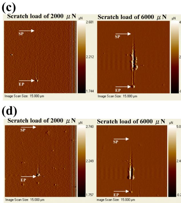
Fig. 1 3D AFM images of the surfaces of the Si-Ge superlattices and the features of the nanoscratch traces zone after annealing (a) RT, (b) 400, (c) 500, and (d) 600 °C. All of these samples had been subjected to ramping loads of 2000 and 6000  $\mu\text{N}$ . We observe pure elastic contact dominated at the low ramped force (2000  $\mu\text{N}$ ), the annealed samples exhibited more pile-up near the middle of the sliding line (6000  $\mu\text{N}$ ) than did the specimen at RT.
