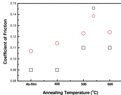
Fig. 3 Distinct critical coefficients of friction of the as-deposited and thermally treated Si-Ge thin films. Scratch techniques are important tools for measuring the effects of adhesion and delamination on the mechanical response.
