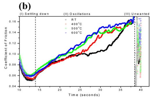
Fig. 2 Typical profiles, determined under ramping loads of (a) 2000 and (b) 6000  $\mu\text{N}$ , of the coefficient of friction with respect to the scratch duration for Si-Ge superlattices that had been subjected to thermal annealing at RT, 400, 500, and 600 °C. The increasing curve is ex-situ to the artificial deformation response during the lateral force load; the possible presence of the elastic/plastic contact translation state is noted.
