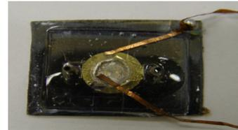
Fig. 6 One example of the assembled micro pump
