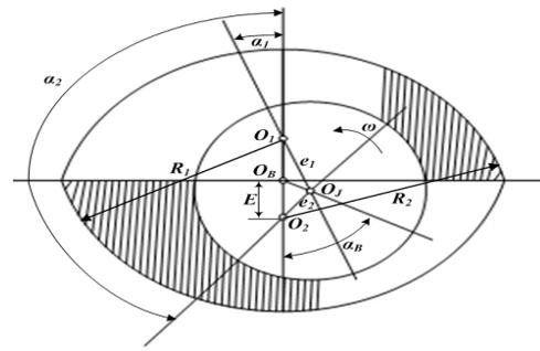
Fig. 1 Elliptic gas bearing system
